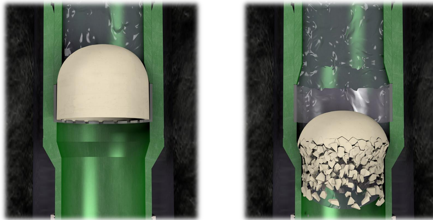
AirLock® casing buoyancy system
